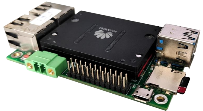
Physical connection with Atlas200 module
